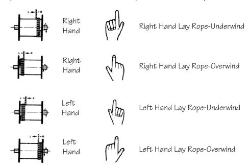
Note: Thumb indicates side of rope anchorage.
